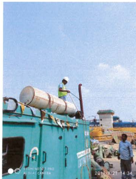
Fig. 13 D—DG stack emission monitoring near main batching plant (DG-4)
