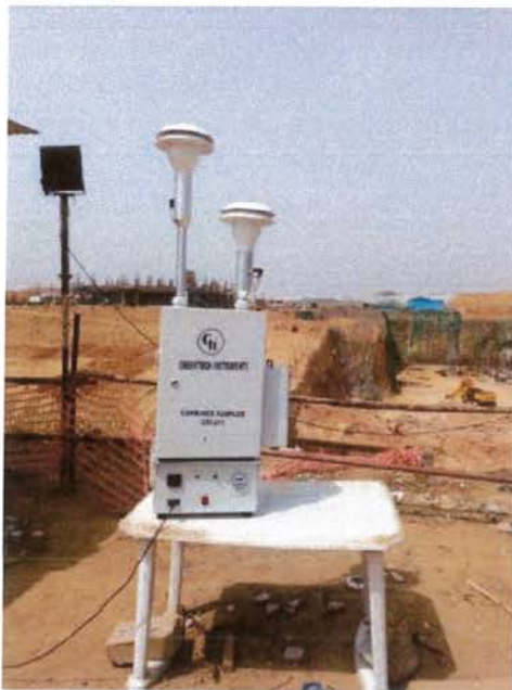
Fig. 13 K & L –Air quality monitoring near Gate 6 (AAQ-1)
