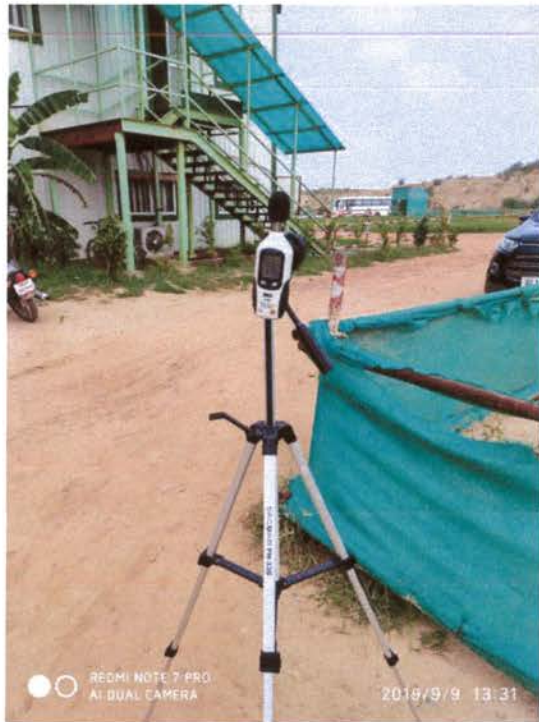
Fig. 13 A—Noise level monitoring near site office (ANQ-2)
