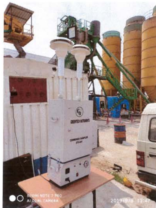
Fig. 13 H–Air quality monitoring near batching plant (AAQ-5)
