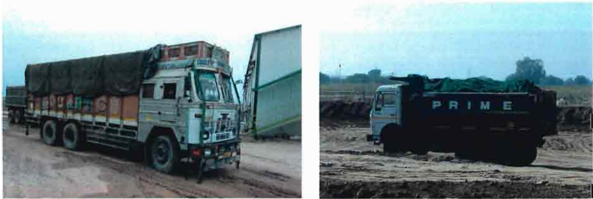
Figure 9: Covered Loaded Vehicle to prevent air pollution
